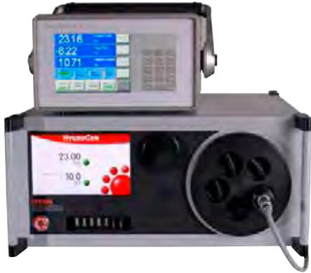
HygroGen2 with external MBW473 dew point reference
